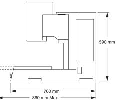
Machine Weight: 100 Kg Crated Weight: 149 Kg
